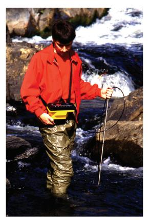
Lightweight, rugged field construction with no moving parts, water resistant electronics, data storage/recall capability, battery operation, and fixed period averaging make it the clear choice in velocity flowmeters.
